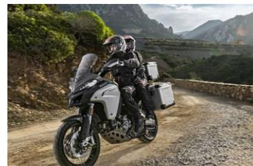
Another challenger to the BMW R1200GS has emerged in Ducati's new Multistrada 1200 Enduro. To make it more suitable for off-road riding, the wheels are now spoked 19/17 inch f/r, a 7.9 inch suspension travel, up from 6.7 inch and 7.9 gal (vs 5.3) fuel capacity for approx 280 miles between fill-ups. So far, only available in Europe, however.
